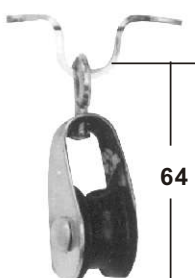
MINI BLOCK AISI 304 For rope \Phi 10 mm plastic sheaves 20x10mm with wire swivel and fender cleat ITEM NO. Weight 017120
