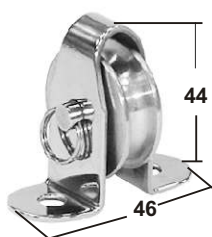
SINGLE LEAD BLOCK AISI 304 For rope \Phi 6 mm brass sheaves 25x6mm 1sheave pin with split ring can take out. ITEM NO. Weight 012029
