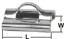
TRACK SLIDE AISI 304 ITEM NO. L mm W mm Weight/g 004311 24 19 8 004312 29 23 10
