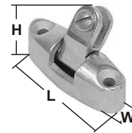
UNIVERSAL DECK HINGE Casted AISI 316 ITEM NO. L mm W mm H mm Weight 009912 70 25 45 180g
