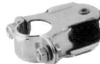
FURLING BLOCK AISI 304 With plastic sheaves to be fitted to pipe 25mm ( \Phi 1" ) stanchion or pulpit ITEM NO. Length mm Sheaves mm Weight 009823 67 25x10 89g
