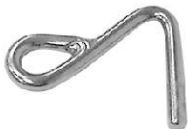
CUNNINGHAM HOOKS AISI 316 with wide flare and parallel eye. ITEM NO. Length Eye dia Stock dia Weight/g mm mm mm 004307 65(2-9/16") 11(7/16") 6(1/4") 31 004308 95(3-11/16") 16(5/8") 8(5/16") 80
