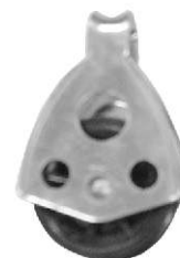
BLOCK AISI 304 For rope \Phi 8 mm plastic sheaves 35x11mm ITEM NO. Weight 019108 31g
