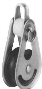
BLOCK AISI 304 For 8mm dia rope brass sheave 30x10mm 1 sheaves ITEM NO. Weight/g 058130 81
