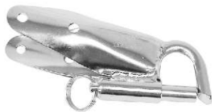
SPI POLE FITTINGS stamped AISI 316 ITEM NO. Weight/g 007996 for tube \Phi 25mm Aluminium tube 96 007997 for tube \Phi 32mm Aluminium tube 98 007998 for tube \Phi 32mm Wooden pole 102
