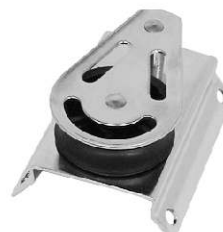
TURNING BLOCK AISI 304 For 10mm dia rope plastic sheaves 35x11mm 1 sheave ITEM NO. Weight/g 012035 70
