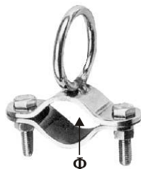
CLAMP WITH RING stamped AISI 304 ITEM NO. \Phi mm Ring Weight/g 009824 25 \Phi 5x30 88
