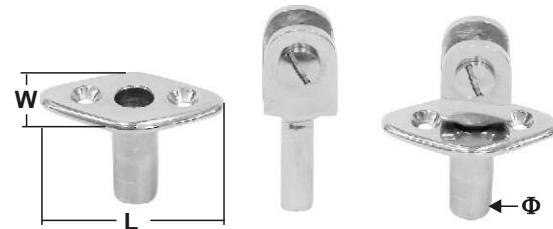
FLUSH BIMINI FITTING casted AISI 316 with jaw and bolt. ITEM NO. L mm W mm 009985 48 29
