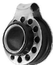
STANCHION ROLLER AISI 304 High speed stanchion roller. This railing-rolls permits to lead the line outside of the railing. The block running in ball bearings. Performed a perfect function and an easy run. Suitably for 25mm railing, line up to 13mm. ITEM NO. Weight/g 012032
