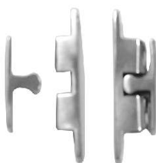
STUD CATCHES casted AISI 316 ITEM NO. Overall size Weight/g 003680 1-3/4"x5/16" (44x8mm) 15 003681 2"x3/8" (50x9mm) 24 003682 2-1/4"x7/16" (57x11mm) 31
