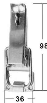
ECCENTRIC LATCH stamped AISI 304 ITEM NO. Thickness Weight/g 008371 1.5mm 64g
