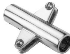
STANCHION SLEEVE casted AISI 316 ITEM NO. Tube O.D. Weight 009777 25mm(1") 392g 009776 30mm(1-3/16") 420g
