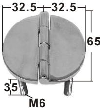
HINGE WITH THREAD precesion casted AISI 316 ITEM NO. WxL mm Thickness mm Weight/g 008625 65x65(2-9/16"x2-9/16") 4 138
