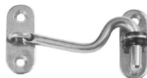
CABIN DOOR HOOK stamped AISI 304 A plastic bushing in the eye prevents assidental unhooking due to vibration
